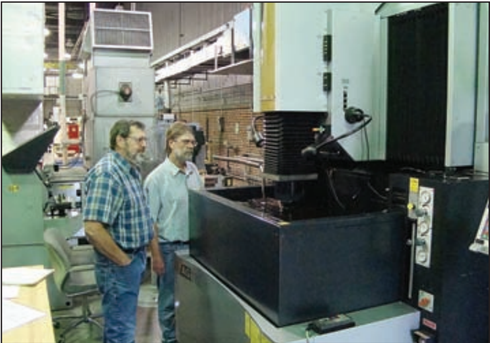
Designer Scott Wieland and Machinist Bill Hopkins observe a new electric discharge machining (EDM) in operation as it is being used to produce balances used in 16T. EDM is a manufacturing process that shapes an object by eroding the material into a specific shape with electrical discharges (sparks).
