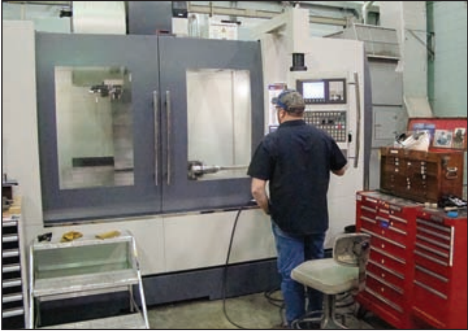
Machinist Gregg Adams operates a new milling machine to produce a part used to collect engine exhaust data. (Photos by Bob Boswell)
