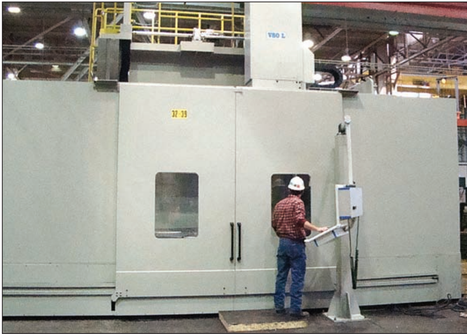
Machinist David Taylor operates the new 80-foot vertical machining center to grind compressor blade assemblies for Plenum Evacuation System. (Photo by Bob Boswell)
