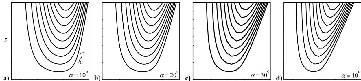
Figure 3. Streamline patterns for  $L=1$  and a)  $\alpha=10^\circ$ , b)  $20^\circ$ , c)  $30^\circ$ , and d)  $40^\circ$ .
