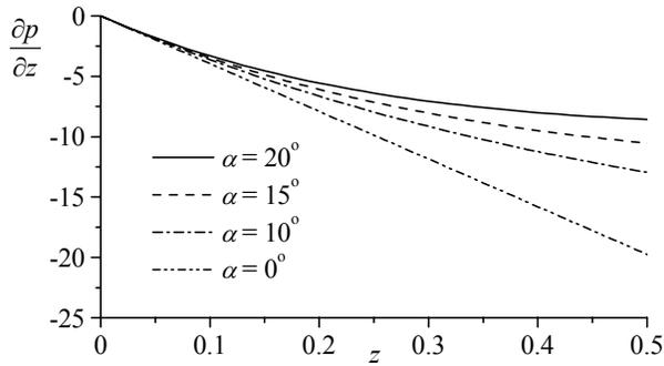
**Figure 8. Axial pressure gradient at several taper angles.**
