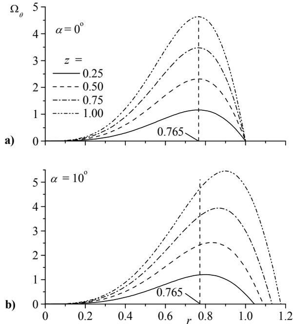
Figure 7. Radial variation of vorticity at several aspect ratios for a)  $\alpha = 0^\circ$  and b)  $10^\circ$ .
