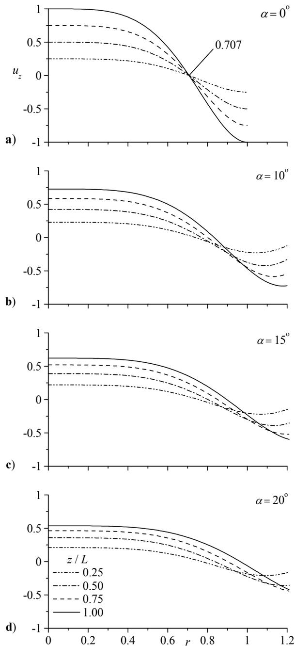
Figure 4. Streamwise velocity at several axial locations corresponding to a)  $\alpha = 0^\circ$ , b)  $10^\circ$ , c)  $15^\circ$ , and d)  $20^\circ$ .
