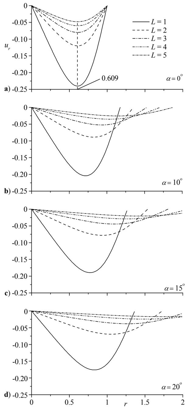
Figure 5. Radial velocity at several axial locations corresponding to a)  $\alpha = 0^\circ$ , b)  $10^\circ$ , c)  $15^\circ$ , and d)  $20^\circ$ .
