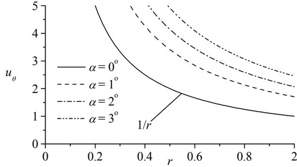
Figure 6. Azimuthal velocity component shown at several taper angles.
