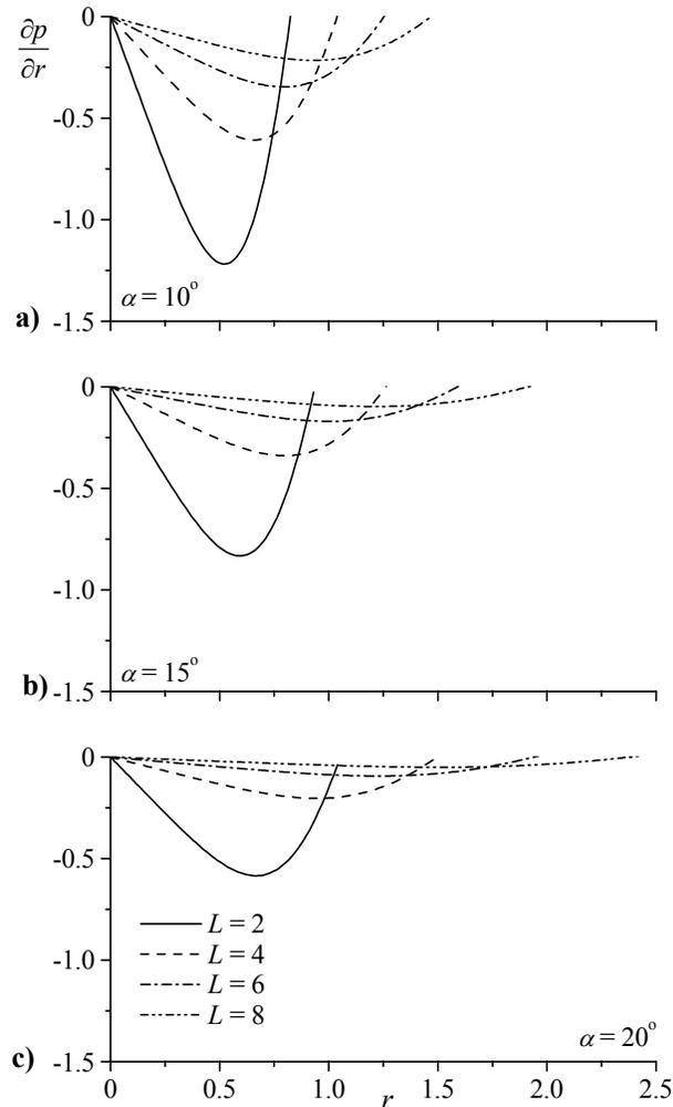
**Figure 9. Radial pressure gradients at several aspect ratios and a)  $\alpha = 10^\circ$ , b)  $15^\circ$ , and c)  $20^\circ$ .**
