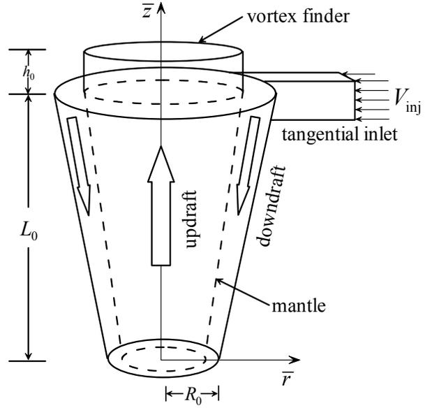
Figure 1. Schematic of typical cyclone separator.
